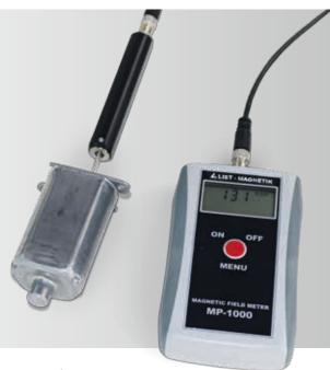
The List-Magnetik MP-1000 magnetic field meter is a handy universal device with externally connectable tangential and axial field probes for the precise measurement of all types of magnetic fields: steady DC fields, alternating AC fields and pulsed fields.
